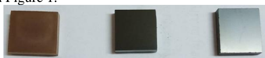
Figure 1. TiSiN, DLC, and TiSiN/DLC coatings on tungsten carbide (Developed by the authors)
