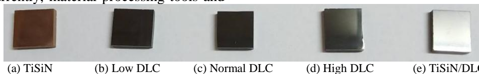
Figure 1. (a) TiSiN, (b) low DLC, (c) normal DLC, (d) high DLC, and (e) TiSiN/DLC coatings on tungsten carbide (Developed by the authors)
